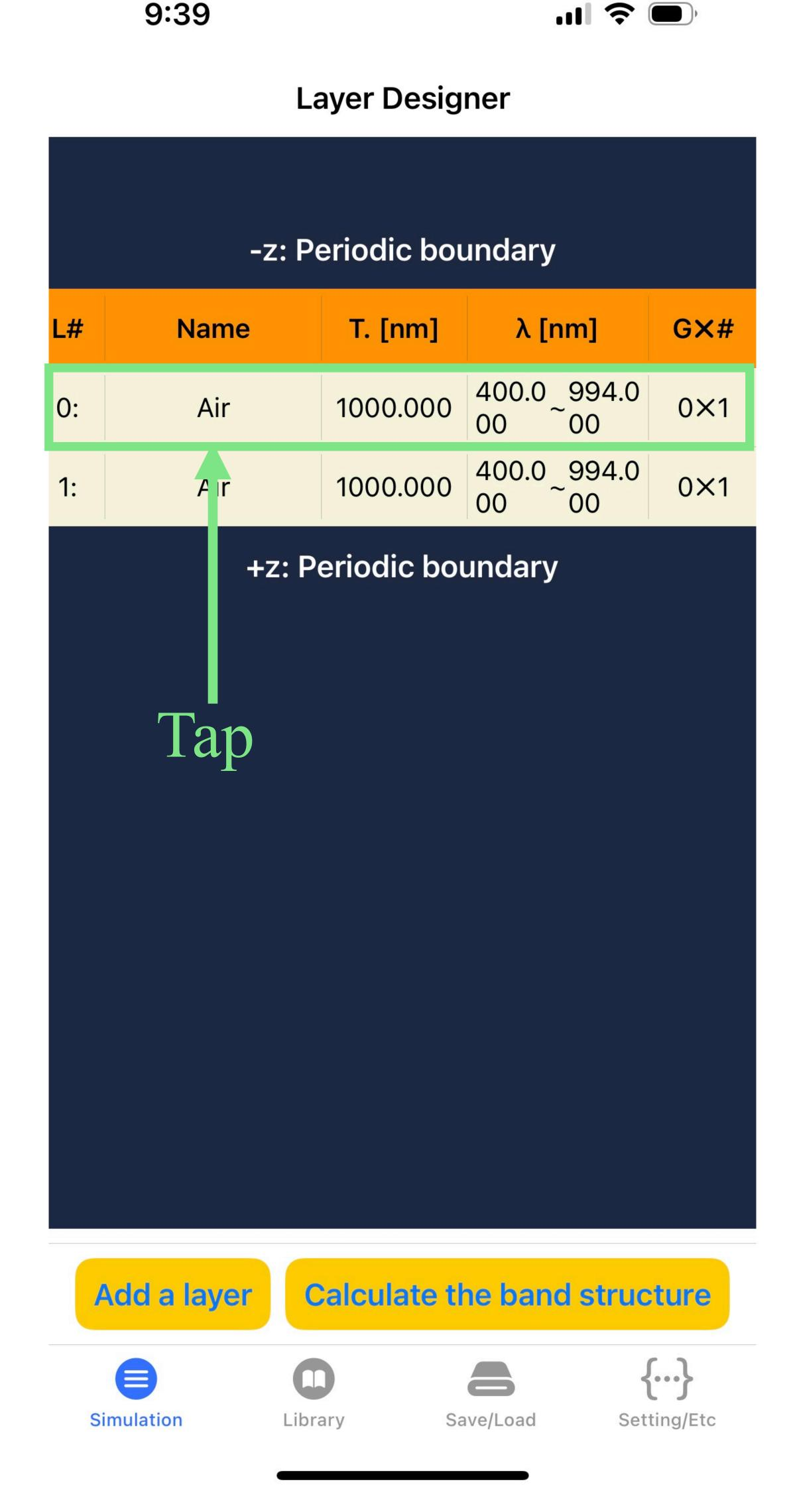
12. Change thickness to 286.36 nm by tapping the "Thickness" field. Then, tap the "Material" button.
