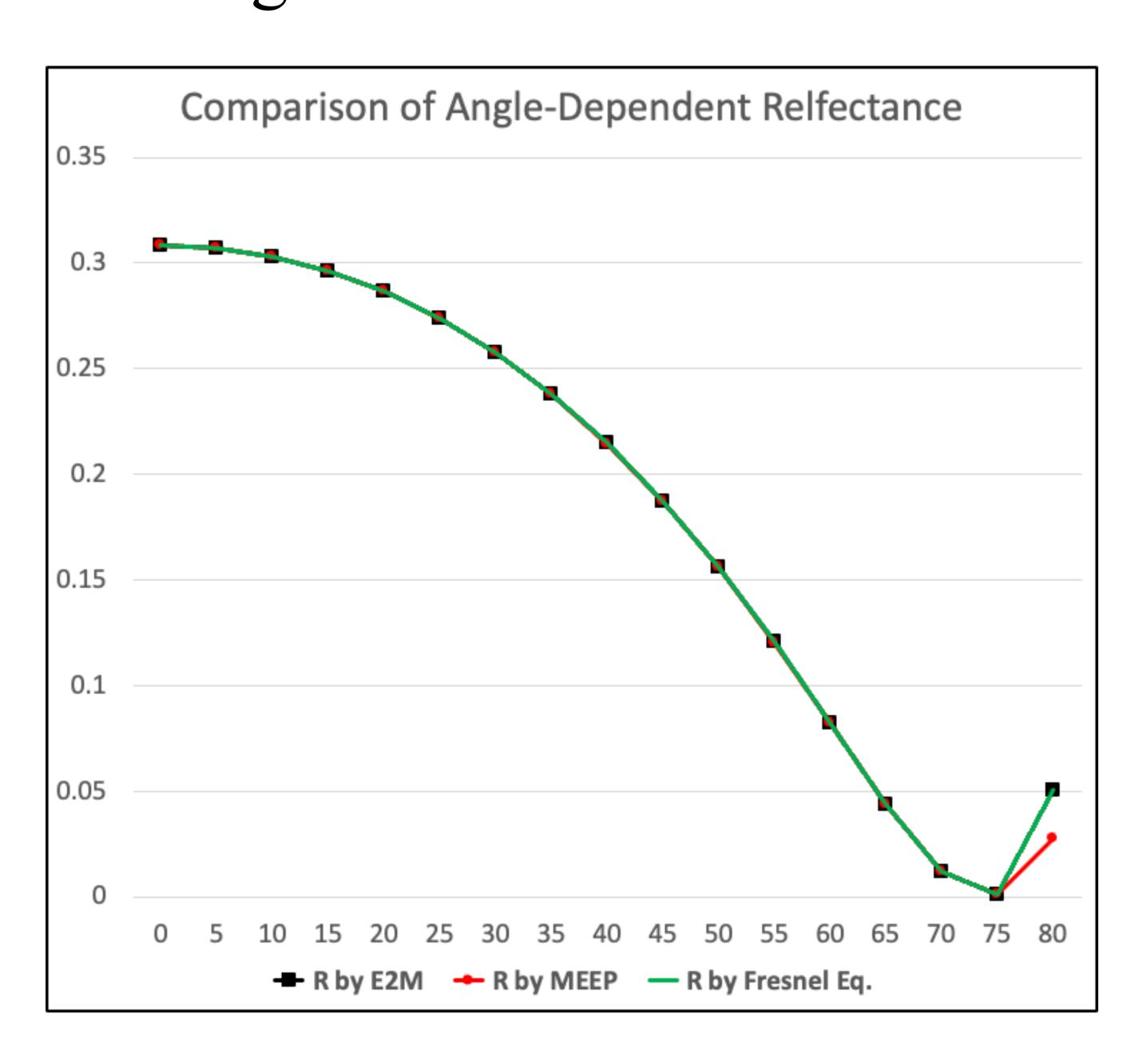
Here, the x-axis means wave incident angles and the y-axis means the reflectance. From 0 to 75 degrees, the results among E2M, MEEP, and the Fresnel equation are identical. However, at 80 degrees, MEEP's result deviates from the other analytical results, at least within the applied simulation conditions. Of course, by pouring computational resources and time, we can get identical results among the three methods.
