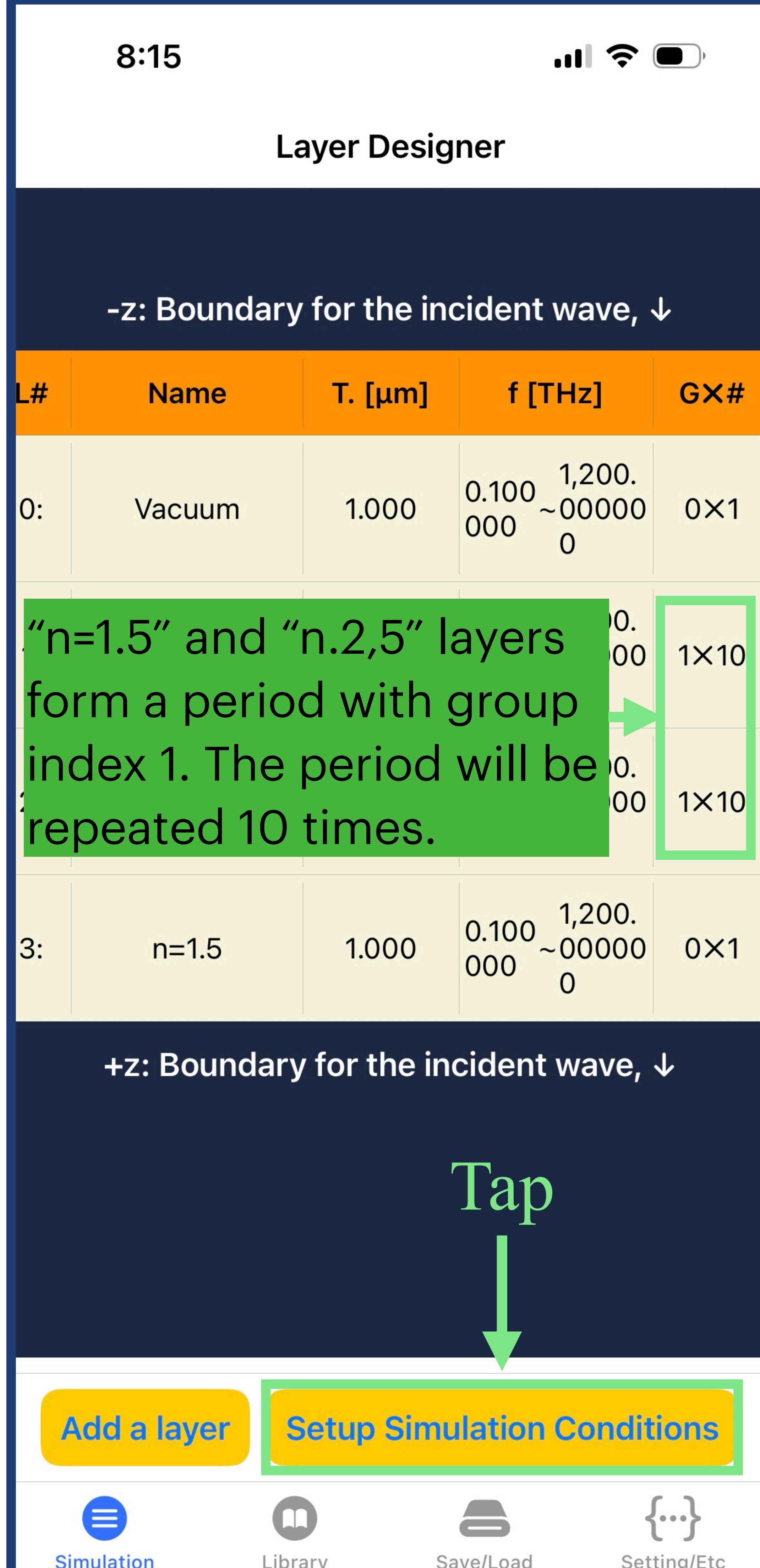
21. Simulating only for  $\theta = 0.0^\circ$  is enough to recalculate the target reference. However, we fill in  $\theta = 0.0^\circ \sim 90.0^\circ$  with  $\Delta\theta = 1^\circ$  to practice more features of E2M. TE polarization is kept to 1.0. After all settings are configured, tap “Perform Simulation” button.
