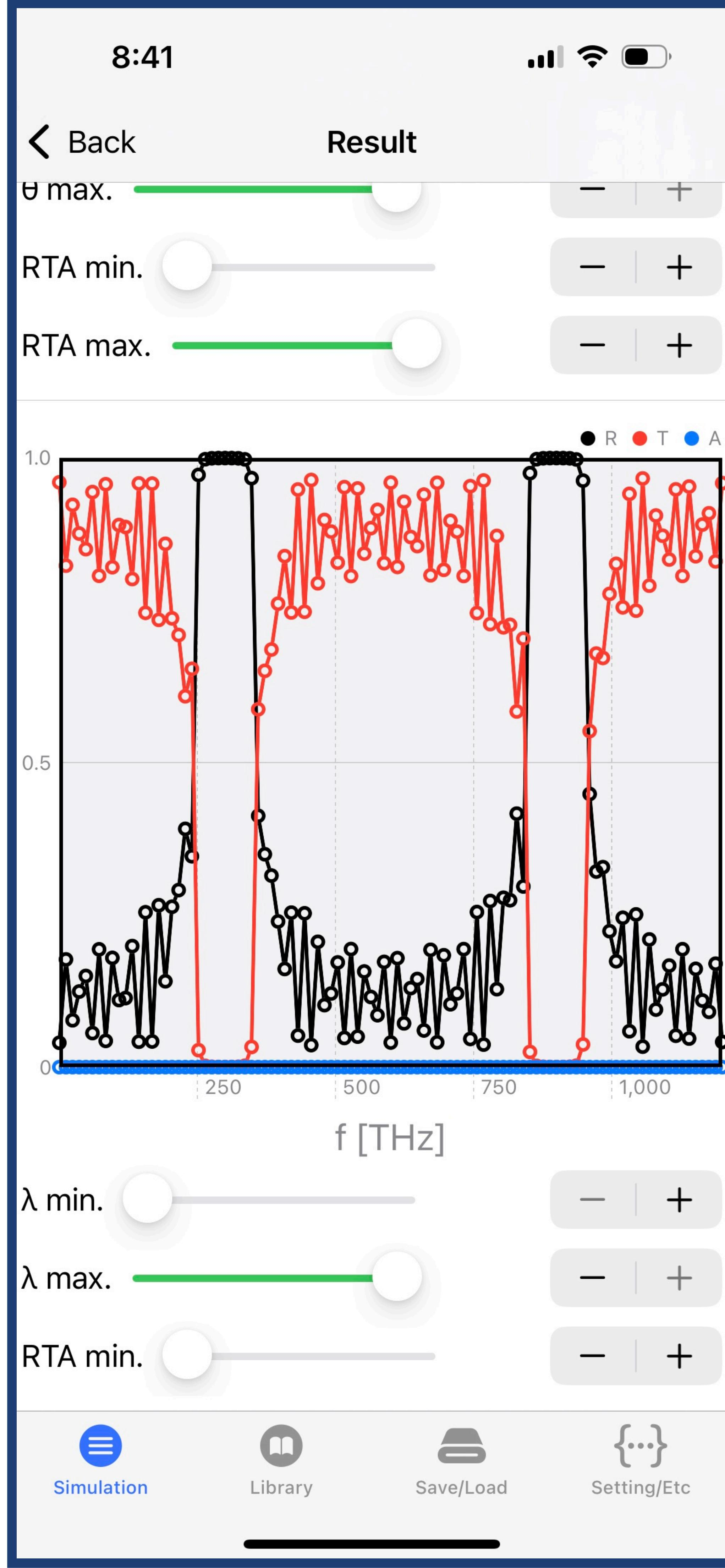
24. By swiping up more, we can see several buttons. Among those, tap “Calculate Field Distribution”. Then,  $E_x$ ,  $E_y$ ,  $H_x$ , and  $H_y$  field distributions are calculated as functions of depth. Before tapping, users may try to control the not-introduced sliders and  $-/+$  buttons freely.
