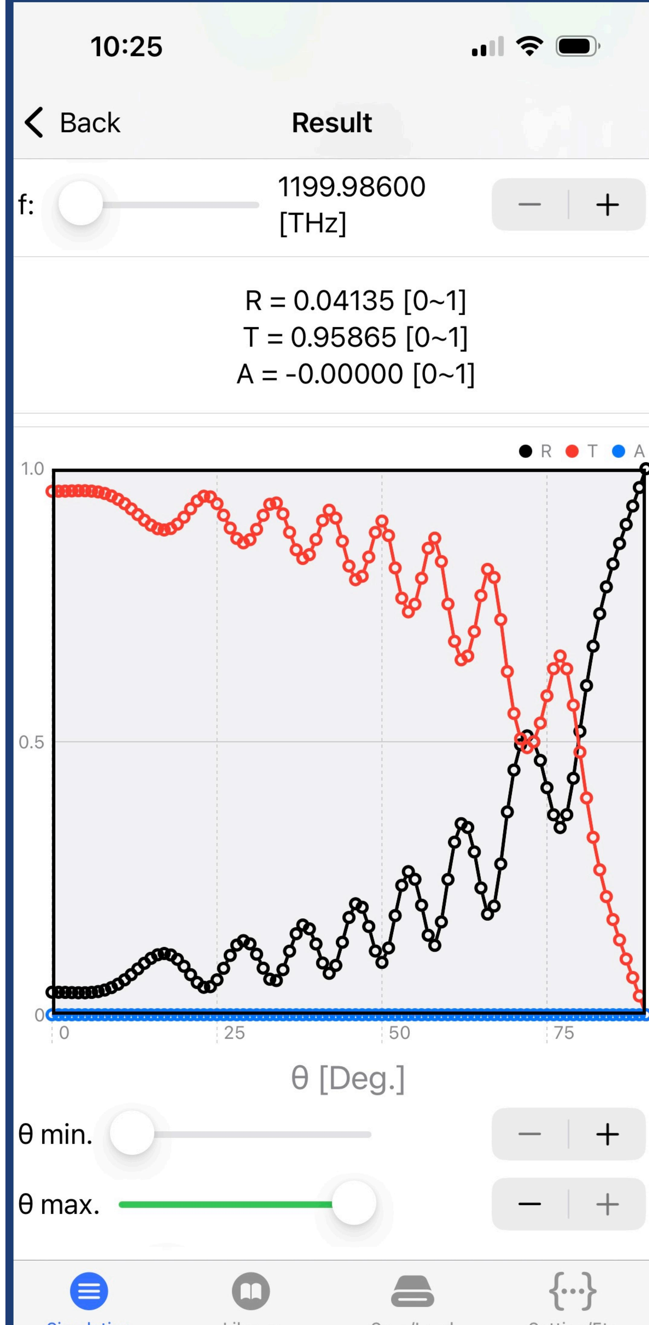
23. By swiping up more, we can see RTA vs. f figure. It shows very similar R result with the reference's lower-side figure. If you want to observe a better matching result, increase the “# of f for RTA” after tapping “Setting/Etc” icon.
