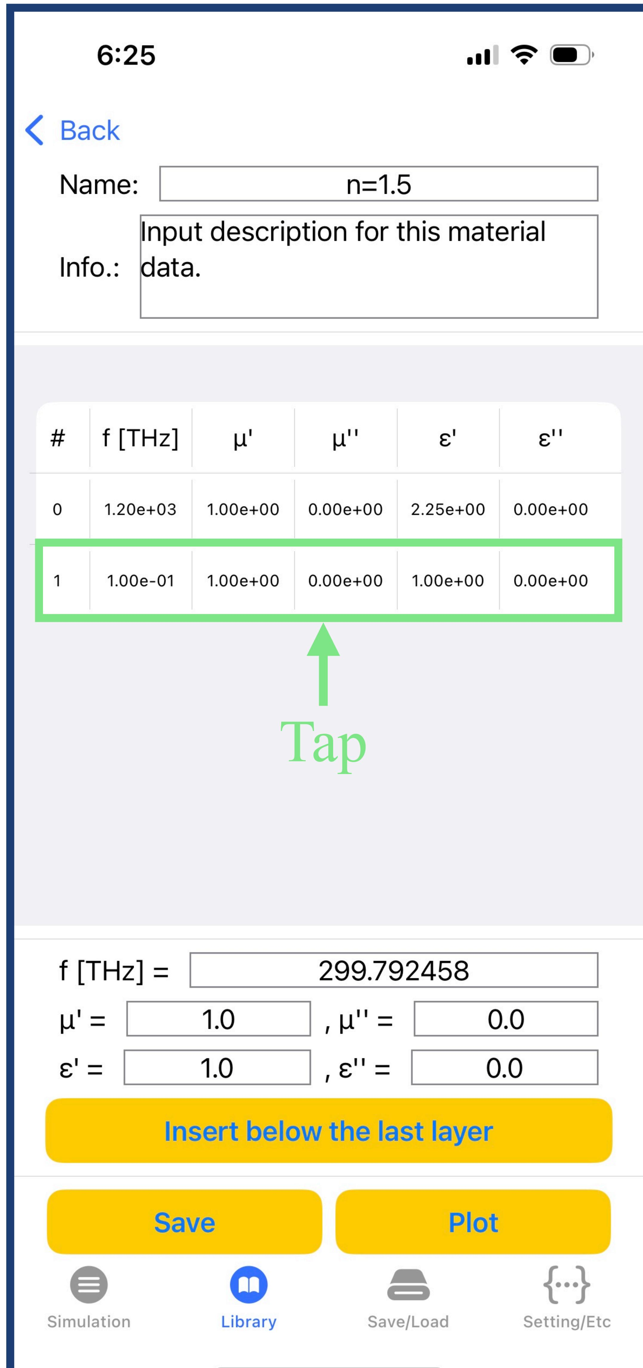
13. Tap the “Save” button to save the user-defined material with  $n=1.5$ . Next, tap the Name field and enter “ $n=2.5$ ”. Next, tap the table’s #0 row. After that, change the value of  $\epsilon'$  to 6.25 and tap the “Apply” button.
