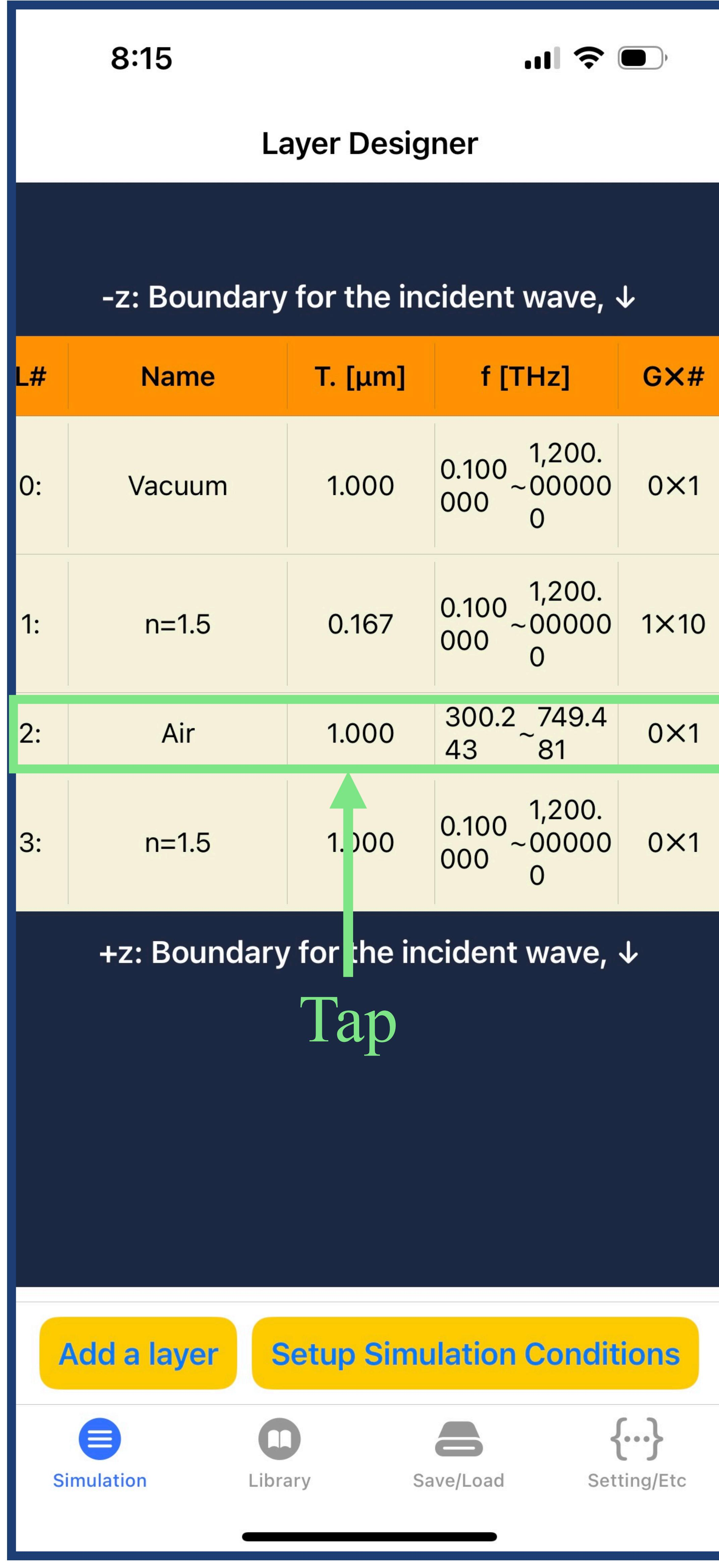
20. When identical group indices exist adjacently right below or above, a periodic structure is internally created. Such a period is repeated as the group repeat number. Tap the “Setup Simulation Conditions” button.
